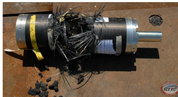
2530 m/s FI – Composite Case (XLDB, no co-oxidizer)
