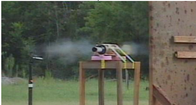
1829 m/s FI – Aluminum Case (XLDB, no co-oxidizer)
