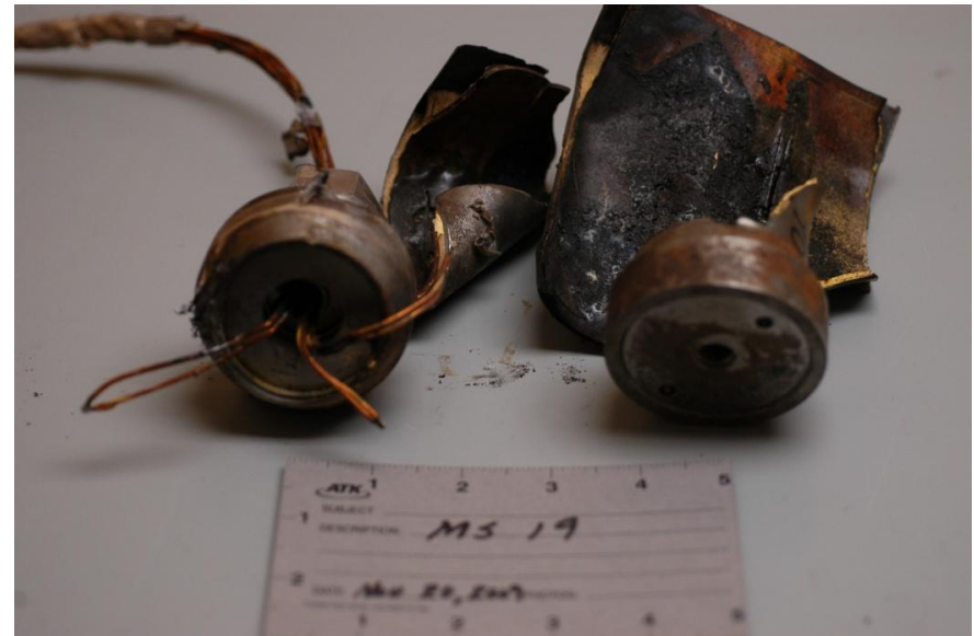
Post-test view of MS (3.3°C/hr)
