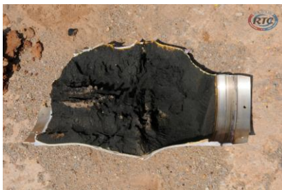
Case fragment with propellant
