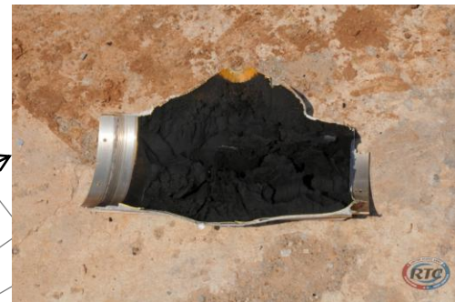
Case fragment with propellant
