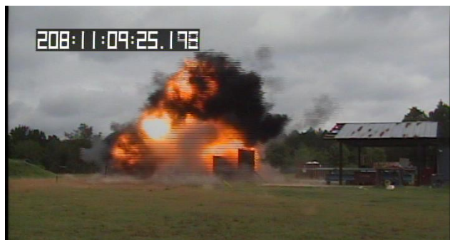
2530 m/s FI – Aluminum Case (XLDB, no co-oxidizer)
